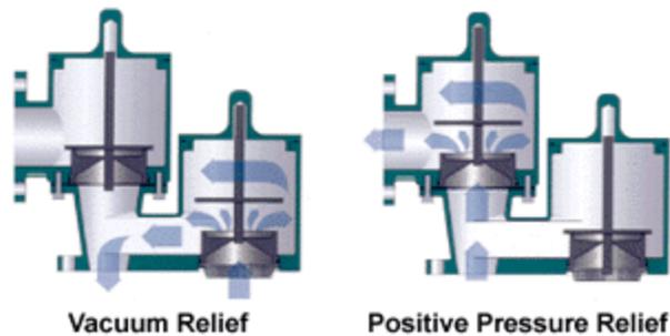
PPS was used by Enardo (an Emerson Electric Company) beginning in 1980 for the seat and pallet of its pressure vacuum vent valves due to the superior performance demonstrated in high content H<sub>2</sub>S applications. These pressure relief valves provide protection against excess positive or vacuum pressure; prevent air intake, evaporative or blanketing product losses; and help contain odorous, hazardous and potentially explosive vapors.
