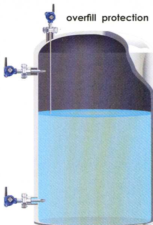
Schematic showing wireless GWR and vibrating fork level transmitters
