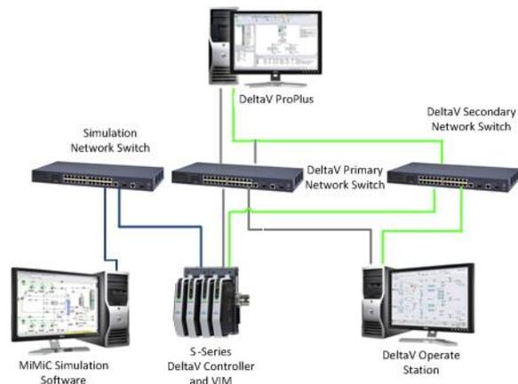
Figure 2: HIL for process simulation and operators training system (OTS)
