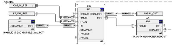
Figure 5: DeltaV – PID control module
