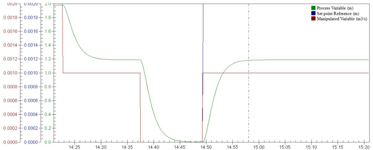
Figure 7: Open loop process response
