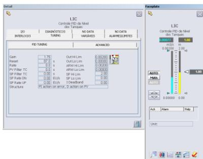
Figure 9: IHM - Process operator interface for the PID Loop
