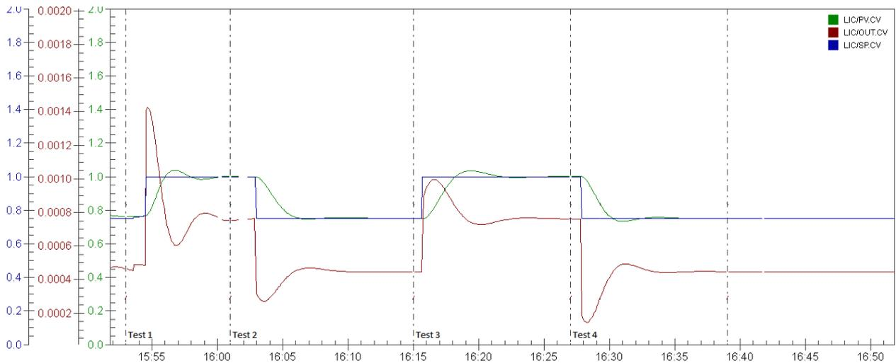
Figure 10: Control loop testing with different PID tuning parameters
