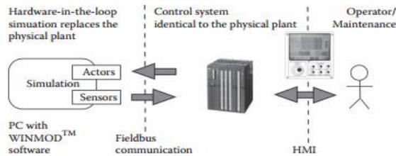
Figure 1: Real-time simulation system: Hardware-In-the-Loop configuration
