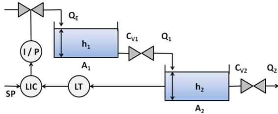
Figure 3: Coupled tanks
