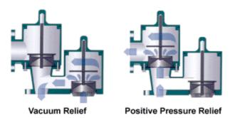
PPS was used by Enardo (an Emerson Electric Company) beginning in 1980 for the seat and pallet of its pressure vacuum vent valves due to the superior performance demonstrated in high content H<sub>2</sub>2S applications. These pressure relief valves provide protection against excess positive or vacuum pressure; prevent air intake, evaporative or blanketing product losses; and help contain odorous, hazardous and potentially explosive vapors.
