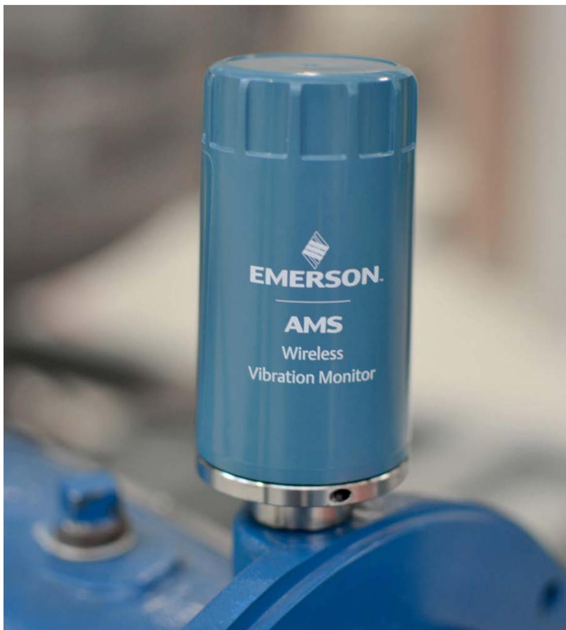
Figure 1: Wireless sensors, like Emerson's AMS Wireless Vibration Monitor, help plants continue to monitor asset health even when short staffed (Image Courtesy: Emerson)
